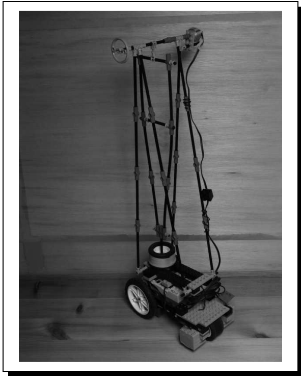
Fig. 1. Bench-top Demonstration. The cart (shown in detail in Figure 2 carries a load suspended by the suspension of Figure 3. The purpose of the controller design is to move the cart between two points whilst suppressing the sway of the load.
