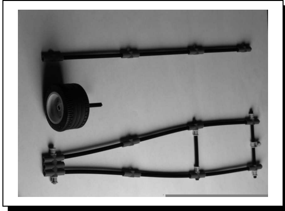
Fig. 3. Load suspension: Detail. Two versions of the load suspension are shown; the left hand version is simple but exhibits resonance effects whereas the right-hand version avoids this problem. The load is also shown; together with the suspension this forms the pendulum.
